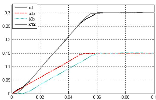
Fig. 9 Translation of the plate with wave control – axis x ( $x_0$  = x-position of the actuator,  $a_0x$  = launched wave in x,  $b_0x$  = reflected wave in x,  $x_{12}$  = x-position of the node 12)
