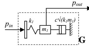
Fig. 4 Scheme of model of the transfer function  $G$
