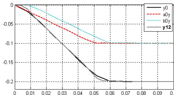
Fig. 10 Translation of the plate with wave control – axis y ( $y_0$  = y-position of the actuator,  $a_0y$  = launched wave in y,  $b_0y$  = reflected wave in y,  $y_{12}$  = y-position of the node 12)
