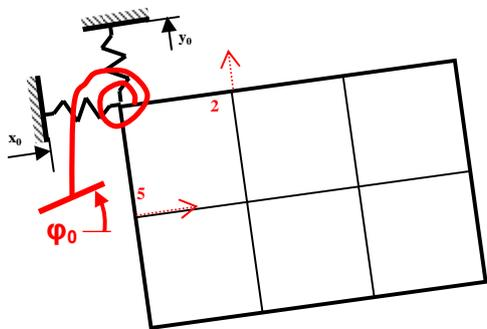
Fig. 11 Torsional actuator for plate rotation
