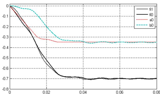
Fig. 12 Time behavior of rotational waves by pure rotation by -0.7 radians
