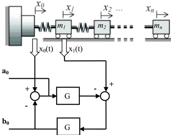
Fig. 3 Scheme of computation of waves  $a_0$  and  $b_0$
