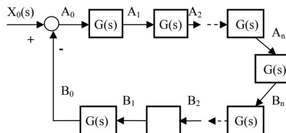
Fig. 2 Wave model of mass system with  $n$  DOFs
