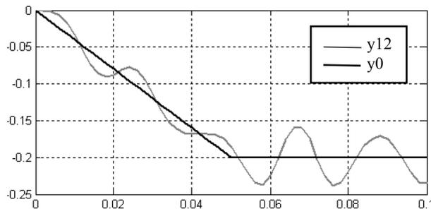
Fig. 8 Translation of the plate (axis y) without the wave control
