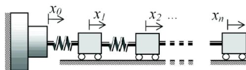
Fig. 1 Model of 1D system with lumped masses
