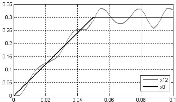
Fig. 7 Translation of the plate (axis x) without the wave control
