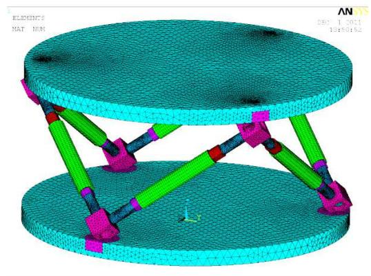
Fig. 4 Platform FEM model grid
