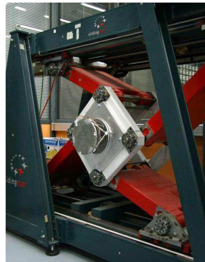
Fig. 1 Sliding Star with active platform
