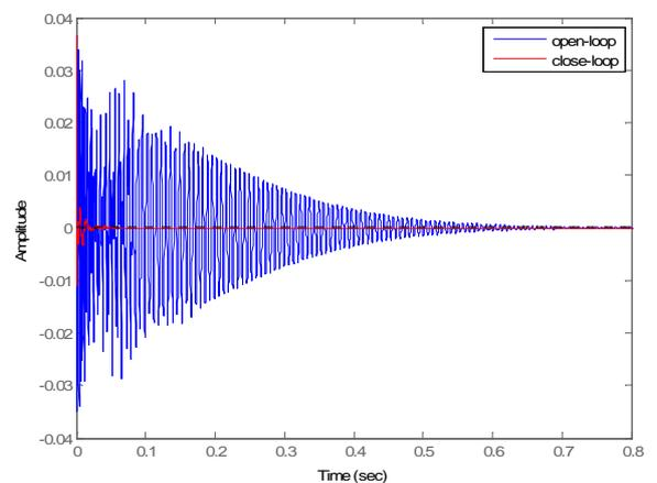
Fig. 11 Step response – from disturbance to acceleration  $X_p$
