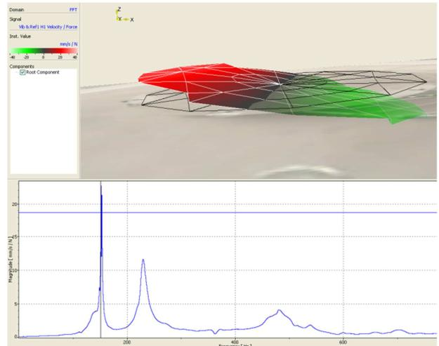
Fig. 14 Modal analysis – Fixed to base frame -151.7Hz
