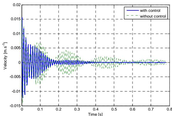
Fig. 17 Experimental results of an active vibration suppression
