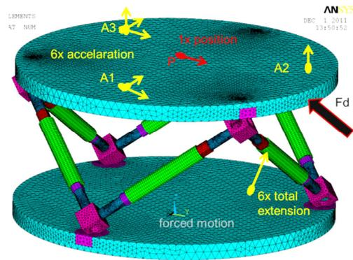
Fig. 7 The choice of inputs and outputs for generalized plant
