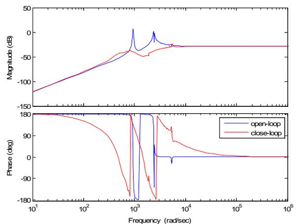
Fig. 10 Transfer function from disturbance to upper base of platform
