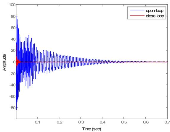
Fig. 12 Dirac impulse – from disturbance to acceleration  $X_p$
