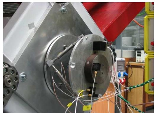
Fig. 16 Active truss structure with accelerometers and additional mass
