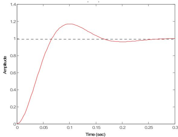
Fig. 13 Step response – from reference position to position  $X_p$
