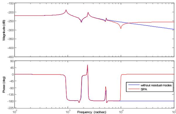
Fig. 8 Transfer function – Fixed to base frame
