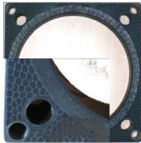
Fig. 2: Cross section of a spindle beam based on the 3D composite structure
