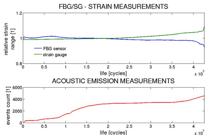
Fig. 9: Comparison of strain range SG and FBG sensor
