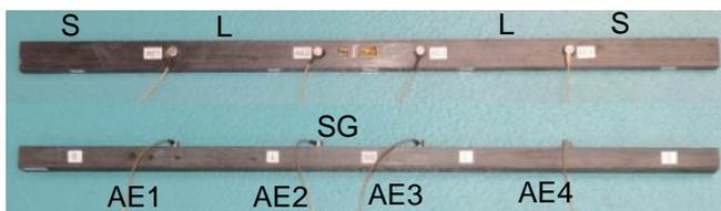
Fig. 7: The specimen for the 4PB test, equipped with the acoustic emission sensors (marked AE) and strain gauge (marked SG). Supports are marked with S, loading points are marked with L
