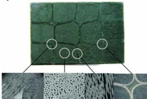
Fig. 3: Details of the parts of the 3D composite structure
