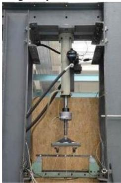
Fig. 5: 4PB experiment configuration
