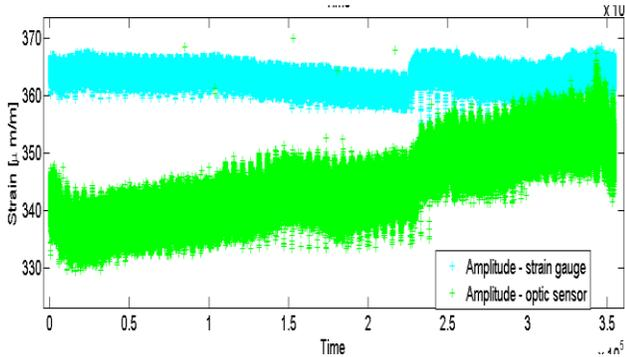
Fig. 10: Comparison of amplitude of strain from SG and FBG sensor (both sensors on surface)
