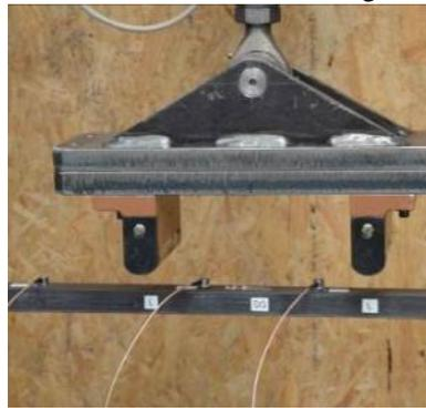
Fig. 6: Detail of the specimen and the active part of the 4PB loading device
