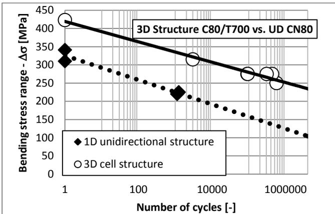
Fig 12: Fatigue properties of the hybrid 3D cell structure CN80/T700
