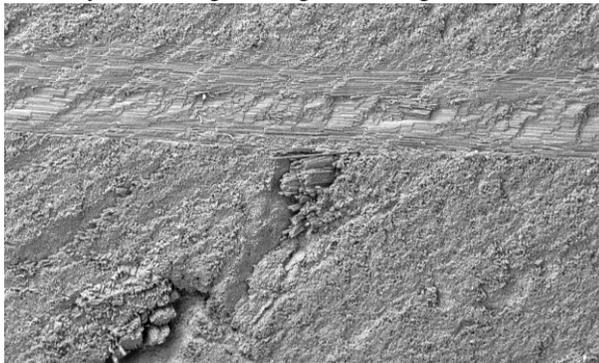
Fig. 17: Growing rapture from core to winding boundary of the sample K63712/T700
