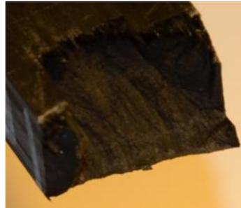
Fig. 16: Rapture area of the sample with high strength fiber K63712
