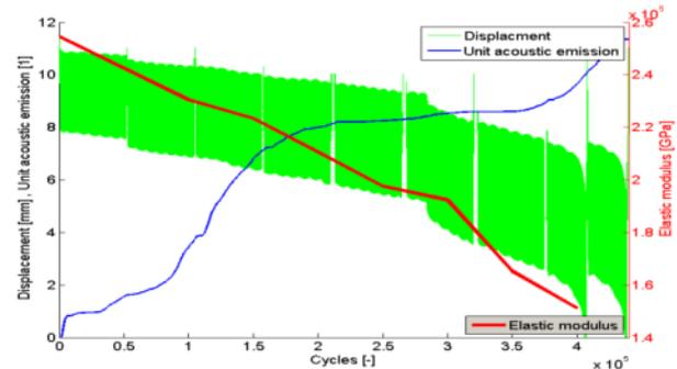
Fig. 8: Deflection of beam, elastic modulus and acoustic event counts during the specimen life (spec. no. 4)
