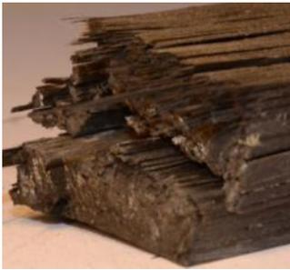
Fig. 15: Rapture area of the sample with high strength fiber T700
