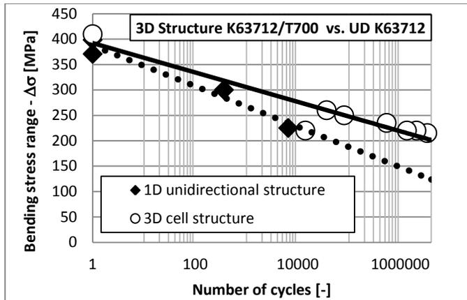
Fig 11: Fatigue properties of the hybrid 3D cell structure K63712/T700
