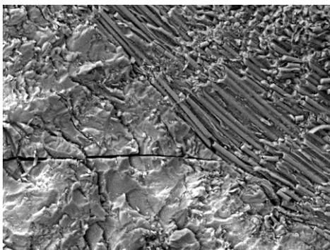
Fig. 18: Growing crack from resin between cell to winding boundary of the sample K63712/T700
