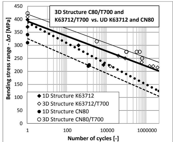
Fig. 13: Comparison of the fatigue properties of the hybrid 3D cell structures - CN80/T700 and K63712/T700
