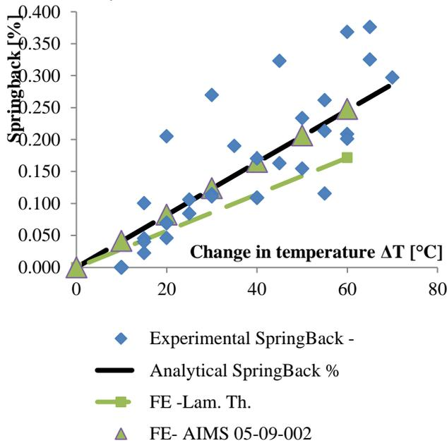
Fig.5. Comparison of analytical, numerical and experimental springforward data
