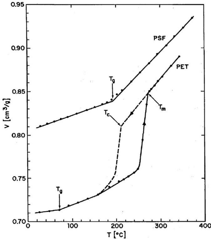
Fig.3. Specific volume of polysulfone (PSF, amorphous) and polyethylene terephthalate (PET, semicrystalline) as a function of temperature during atmospheric pressure [7]
