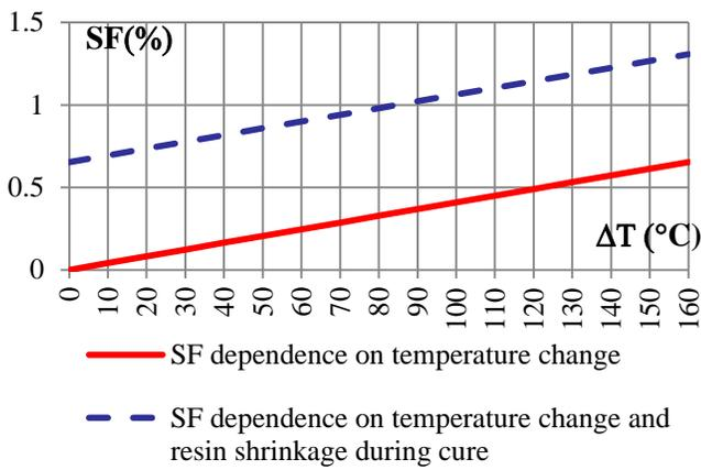
Fig.4. Relationship between the springforward (with and without calculating the resin shrinkage) and the change in temperature
