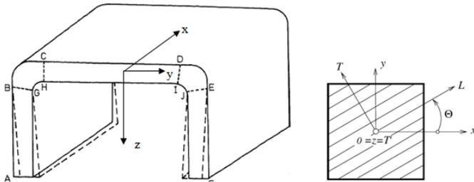
Fig.1. Distortion of moulded U-section [4]
