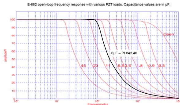
Fig. 9: E-662 Servo unit transfer function [14]
