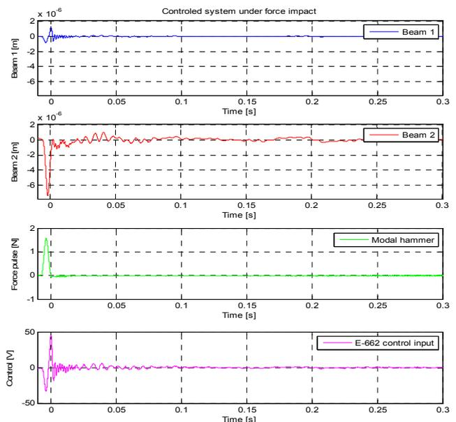
Fig. 18: Controlled System: Beam 1 – force impact
