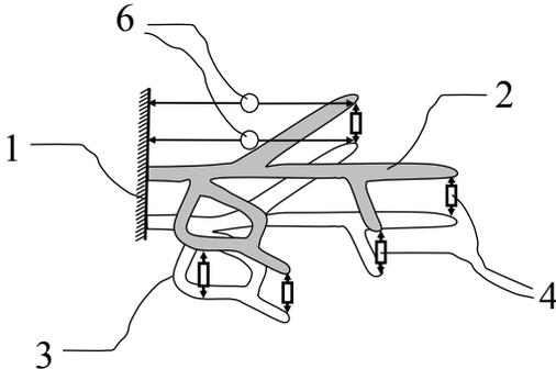
Fig. 1: Concept of mechatronic stiffness from auxiliary structure
