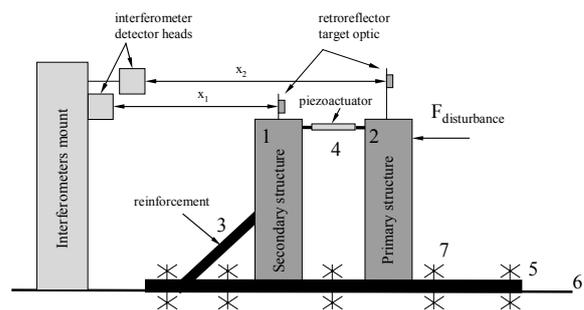
Fig. 5: Experimental concept design
