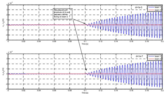
Fig. 16: Disturbance rejection – time domain
