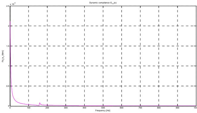
Fig. 13: Decrease of dynamic compliance of beam 1 by active control
