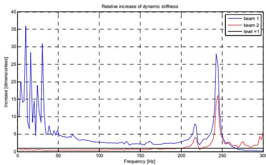
Fig. 19: Dynamic stiffness relative increase - controlled versus uncontrolled system
