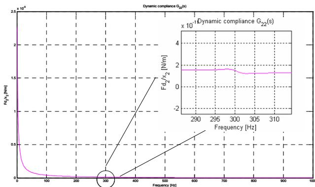
Fig. 14: Decrease of dynamic compliance of beam 2 by active control
